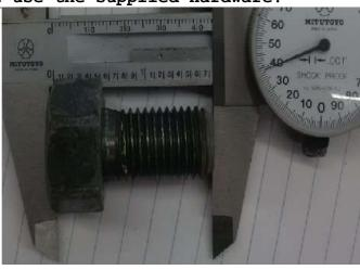
We supplied longer bolt with washer & lock washer, please use this new gold hardware to install the spacer to the axle. Recommend adding Loctite to the bolt, even if there lock washer
